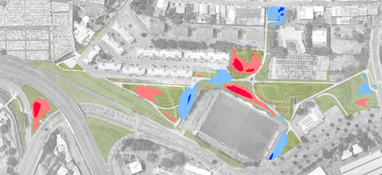
Figure 21: even though construction will move 10.000 cu.m of soil, in the end there is earthwork balance. Earth grading is required for slope stabilisation, creating conditions for human use, designing for water retention and infiltration, creating areas for active recreation. In red cut areas, in blue fill areas.
