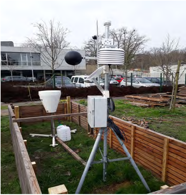
Figure 4: The meteorological station at Stendhal Middle school in the Northern district of Nantes, France. The station is equipped with all necessary sensors to evaluate thermal comfort: air temperature and air humidity sensors, an anemometer for wind speed and direction, and a black globe thermometer to evaluate the mean radiant temperature. The Universal Thermal Climate Index (UTCI) computed with this meteorological station between February 2022 and January 2023, is shown on the right, with the average values per month and per hour of the day.
