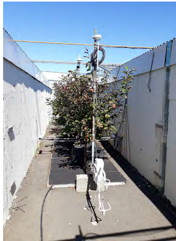
Figure 5. Left: Scale model of a canyon street with North-South orientation to study urban overheating and the impact of street trees on human thermal comfort. The trees are well-watered ornamental apple trees, located on the central axis of the street. Right: The thermal stress evaluated in this street with microclimate measurement and the Universal Thermal Climate Index (UTCI), during a typical summer sunny day, with the different thermal stress categories: no thermal stress (9 to 26 °C UTCI, green), moderate heat stress (26 to 32 °C UTCI, yellow), strong heat stress (32 to 38 °C UTCI, orange), very high heat stress (38 to 46 °C UTCI, red). (adapted from Mballo et al., 2021)
